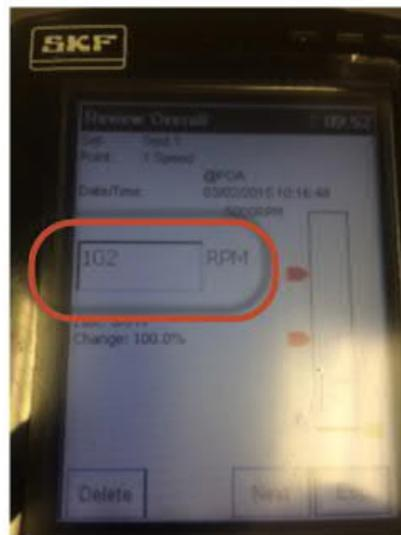
Figure 2. Manually-entered RPM value as 102 in Microlog Analyzer
