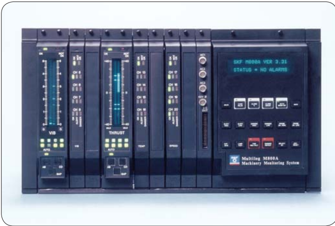
Fig. 4. SKF M800A monitor keeps track of turbine r/min, bearing clearances, shaft vibration, thrust, etc.
