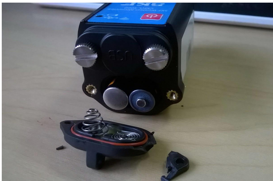
Figure 1: Wireless MicroVibe unit showing battery cover with broken ear
