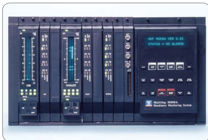
Fig. 1. The SKF M800A programmable machinery monitoring system monitors radial vibration, axial position, temperature and speed on an acetylene screw compressor driven by a 4 500 hp motor.
