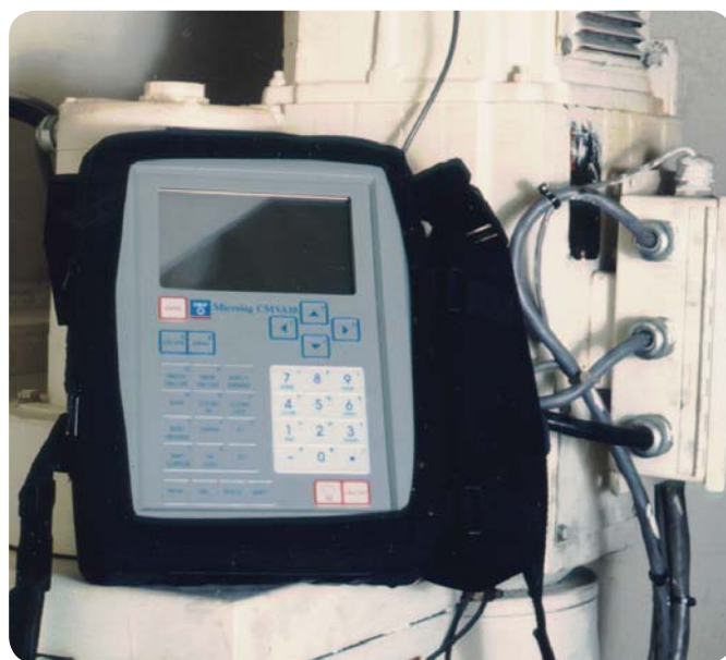
Fig. 1. SKF Microlog data collector/analyser equipped with SEE technology to detect early bearing damage. It will operate as a stand-alone frequency spectrum analyzer or a data collector for PRISM 4 – SKF's specialized software for in-depth historical analysis of preventative maintenance data.
