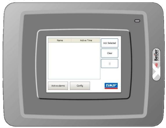
Table includes name, state, alarm activation time and acknowledge time. It will display all alarms including all acknowledged alarms.
