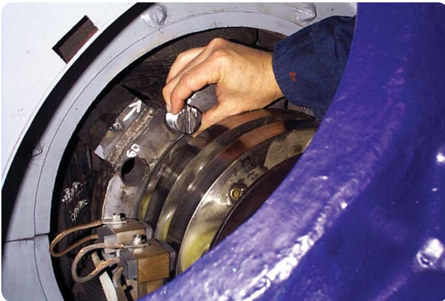
Fig. 2. Adding a trim weight to the field balance ring. Note the slow speed balance stand weight welded on top of the balance ring in order to keep the balance ring holes open for trim balancing.
