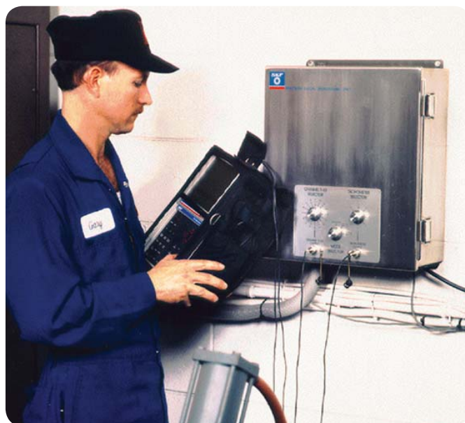
Fig. 1. Both the SKF Local Monitoring Unit, a 32 channel NEMA enclosed vibration monitor, and the SKF Microlog portable data collector analyzer are used to confirm mechanical and electrical problems.
