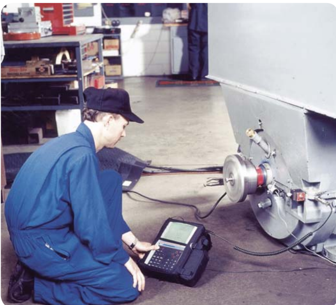
Fig. 2. Gary Herr, vibration analyst at Demaria Electric, uses the SKF Microlog balancing wizard to determine unbalance.
