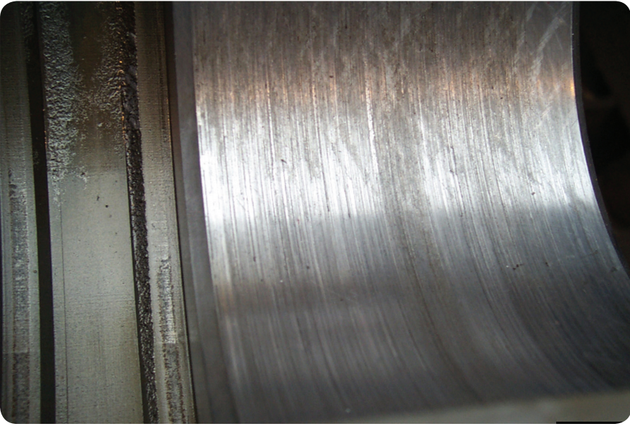
Figure 3. Absorption fan, bearing damage.
