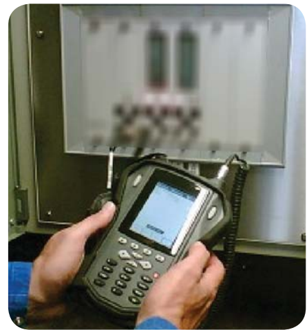
Figure 3. SKF Microlog GX Series collecting measurements from a protection system.
