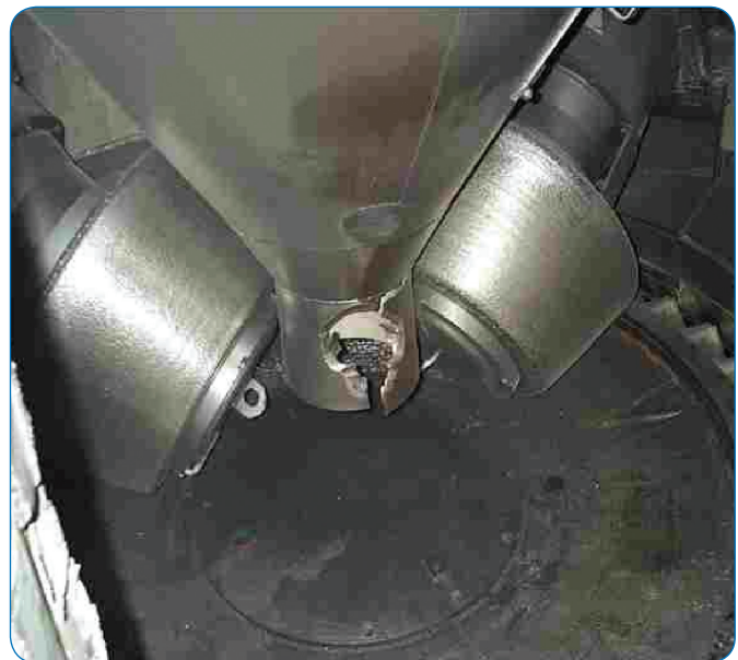
Figure 11. The damaged center feed pipe.
