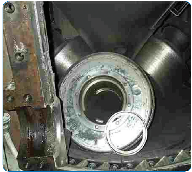
Figure 10. The failed bearings.
