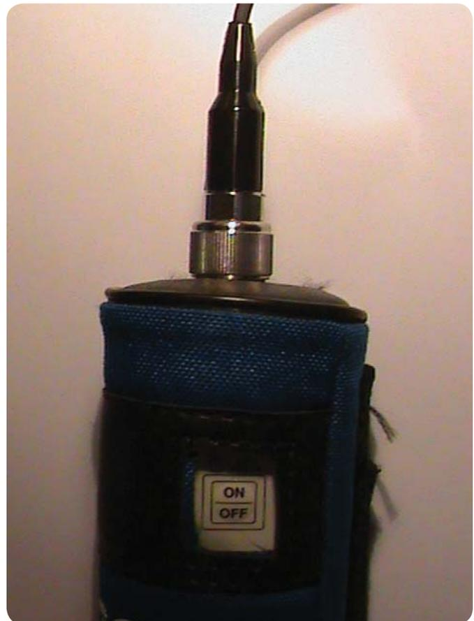
Fig 14. Accelerometer attached to the portable calibrator.
