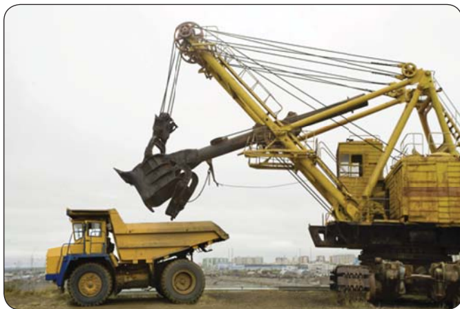
Fig. 1. Example of machines where the rotational direction is important during the vibration measurement.
