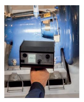
The SKF TKRS 41 is designed for general maintenance tasks and with its standard operating mode, it is streamlined for fast and straightforward usage. The professional mode can be activated for more demanding applications, for example when enhanced input signal modification is needed to trigger the stroboscope with machine signals. For more convenience during inspections, the "SLOW" function can be used to examine all parts of the rotating machine in slow-motion.
