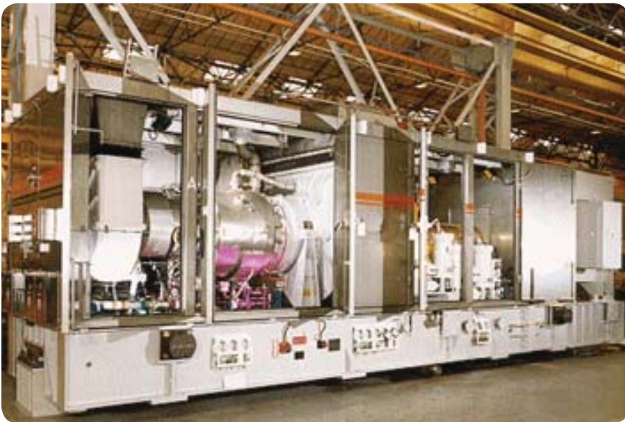
Fig. 3. Aeroderivative gas turbine.
