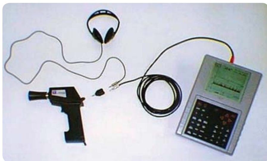
Fig. 1. Components for connecting the Inspector 400 ultrasonic probe to the SKF Microlog CMVA 60.
