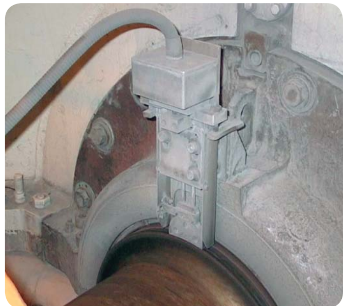
Figure 3. Pendulum probes. Figure 4. Pendulum probe installation.
