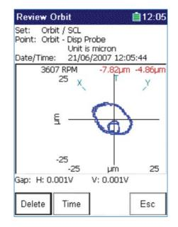
On the SKF Microlog Analyzer GX, the precession of the orbit loops can be examined by using continuous acquisition mode. Alternatively, after unloading to SKF @ptitude Analyst, the orbit can be viewed one rotation at a time to see how the loops change.
