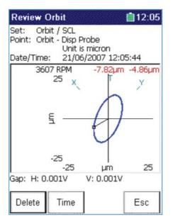
Note that in the SKF Microlog Analyzer GX, filtered orbits are only supported in NonRoute, and any harmonic from 1X to 8X can be viewed. In SKF @ptitude Analyst, orbits are stored in unfiltered mode, but can optionally be viewed with a 1X, 2X or 3X filter applied.
