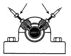
For NonRoute Orbit measurements, the sensors are assumed to be placed at  $0^{\circ}$  (X – CH1) and  $90^{\circ}$  (Y – CH2), and so the actual shaft motion may be rotated relative to that shown on the screen.
