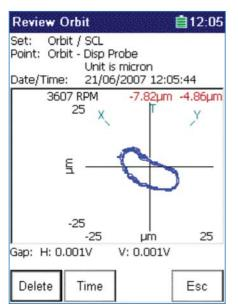
The orbit of a shaft experiencing oil whirl will show a secondary loop that moves around independently of the unbalance loop, as it is not synchronous with rotation.
