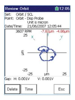
Misalignment will add significant levels of vibration to the shaft at once-per-revolution signal, and will show vibration at 1X harmonics. The once-per-revolution component from misalignment will not be in phase with the unbalance component. The effect is to make the orbit plot less circular and more elliptical or even non-elliptical (i.e., banana-shape or figure-eight pattern).
