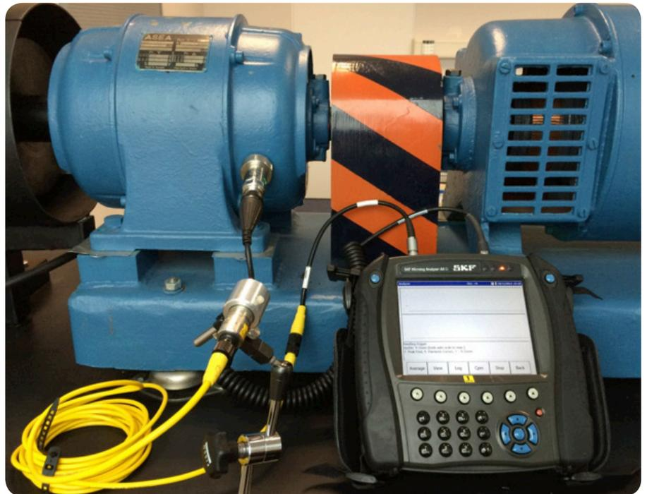
*Order Tracking Measurements with the SKF Microlog Analyzer series and SKF @ptitude Analyst software.*
