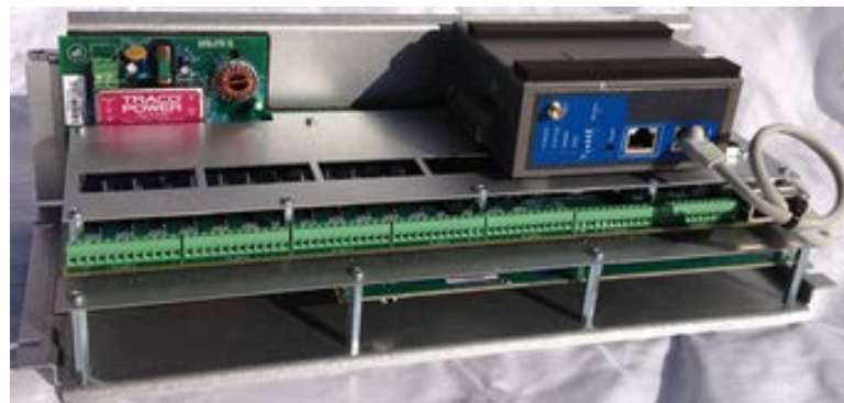
Figure 1 - 3. SKF Multilog On-line System IMx-B, Inside.
