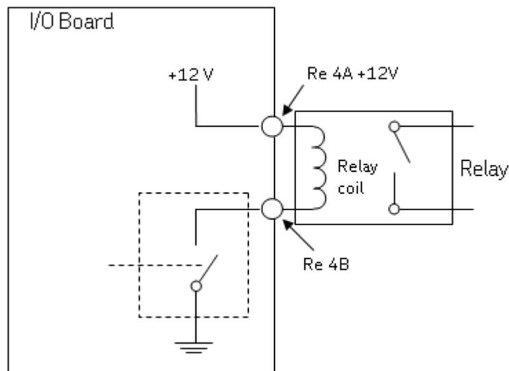
Figure 3-16: Relay open collector driver showing alarm inactive
