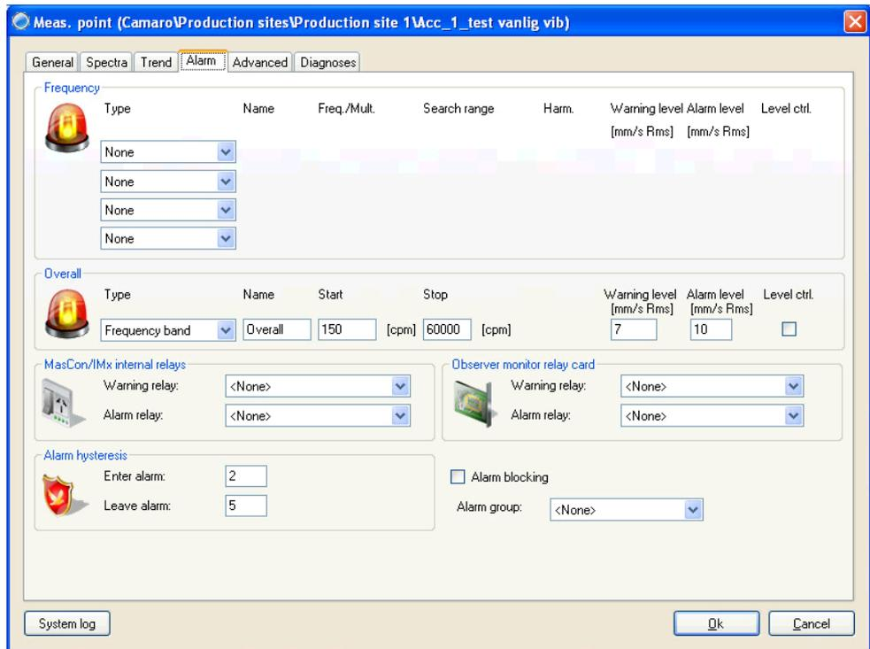
Figure 3-13: Example of Overall in Alarm setting for vibration measurement point
