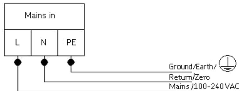
Figure 2-9: Power cable connection
