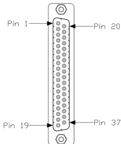
Figure 3-14: Pin numbers for 4-20 mA 37-Pin D-sub (female)
