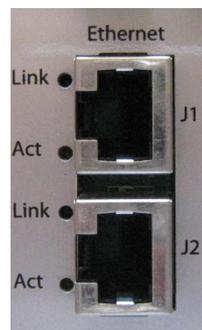
Figure 2-10: IMx-T Ethernet ports
