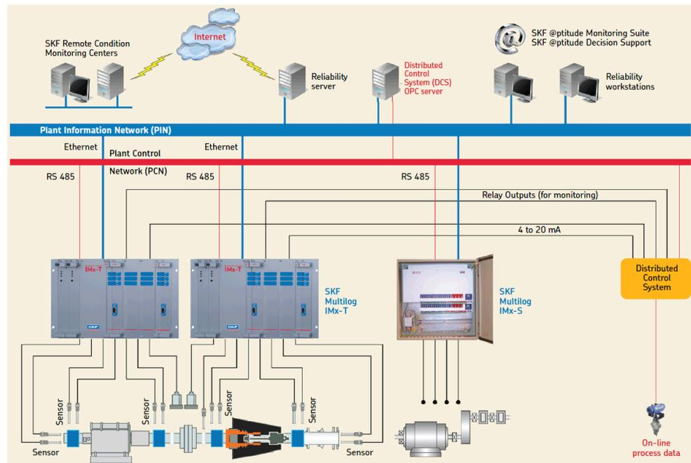
Figure 2-6: Example of typical non-hazardous area installation
