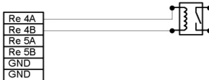
Figure 3-15: Relay driver connection of one output
