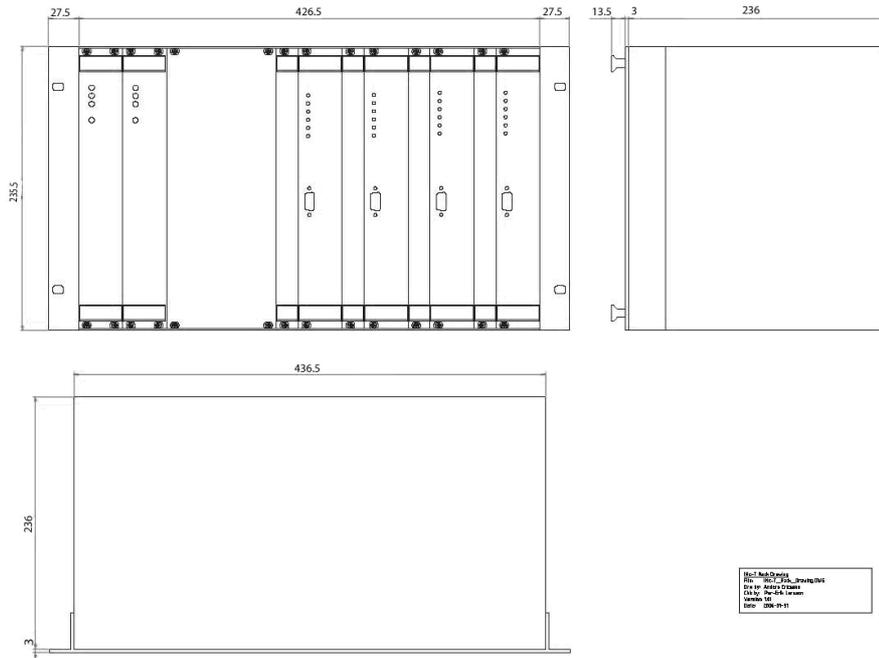
Figure 9-18: IMx-T rack drawing with dimensions
