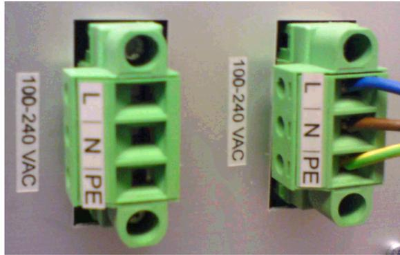
Figure 2-8: Power connection inlets, one for each redundant power supply
