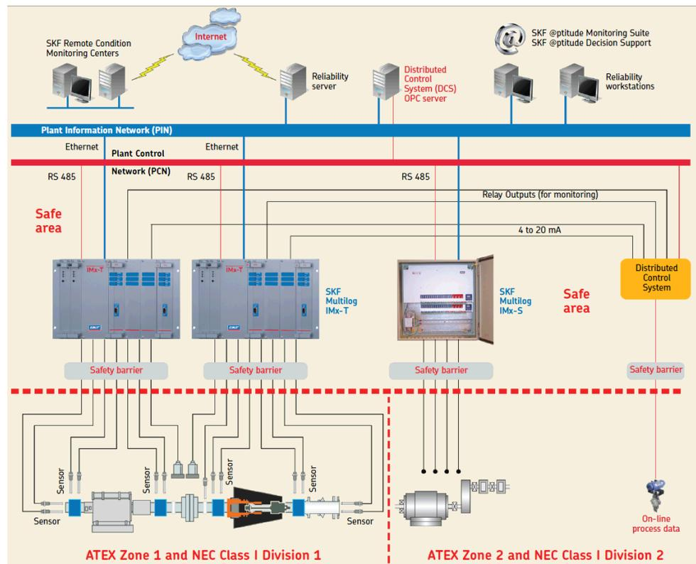
Figure 2-7: Example of typical hazardous area installation
