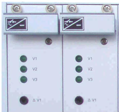
Green LEDs **V1**, **V2** and **V3** of each slot indicate the power presence.
