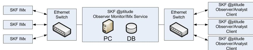
Figure 1-1: System overview, IMx-T with @ptitude Observer/Analyst
