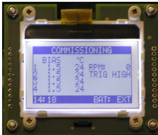
Figure 5 - 5. Commissioning Mode Display.
