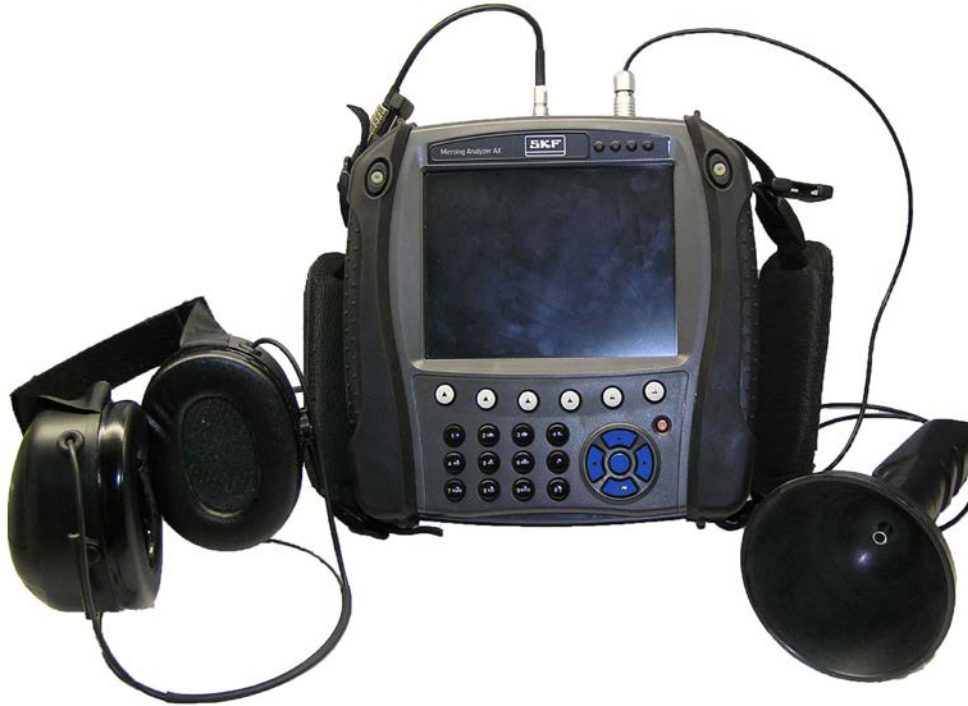
Figure 11 – 2. Microlog with Idler Sound Monitor Module, Earphones, and Microphone with Parabolic Reflector.
