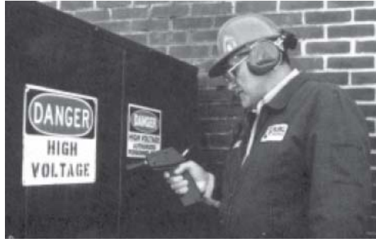
Figure 8. Test switchgear, transformers, etc., for arcing, tracking, and corona.
