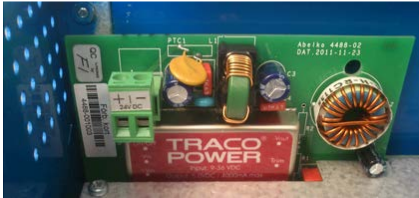
Figure 2 - 2. 24 V DC Power Supply Terminals.
