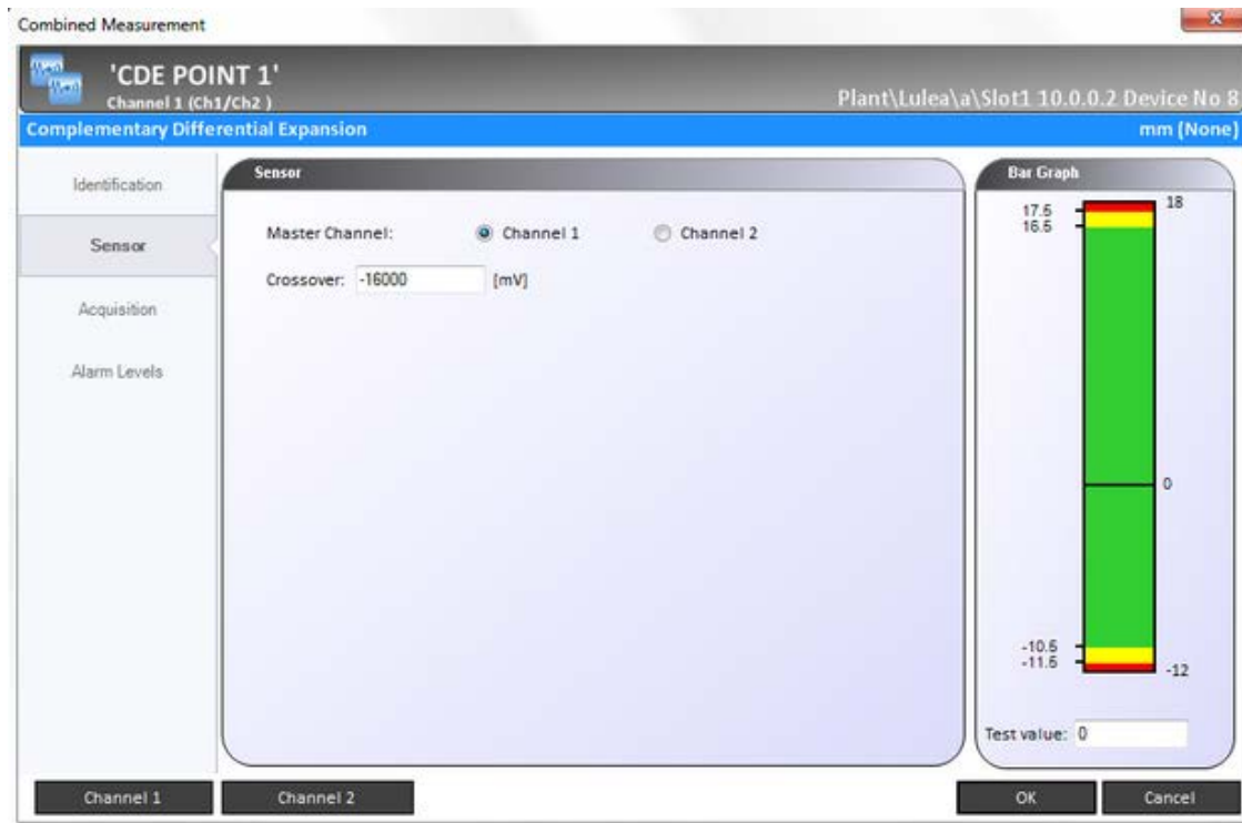
Figure 2 - 124. Selecting the Master Channel and Crossover Voltage.
