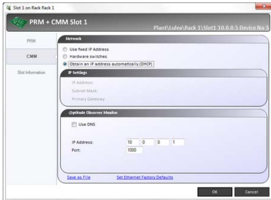
Figure 2 - 80. Using DHCP to Automatically Assign the Slot IP Address.
