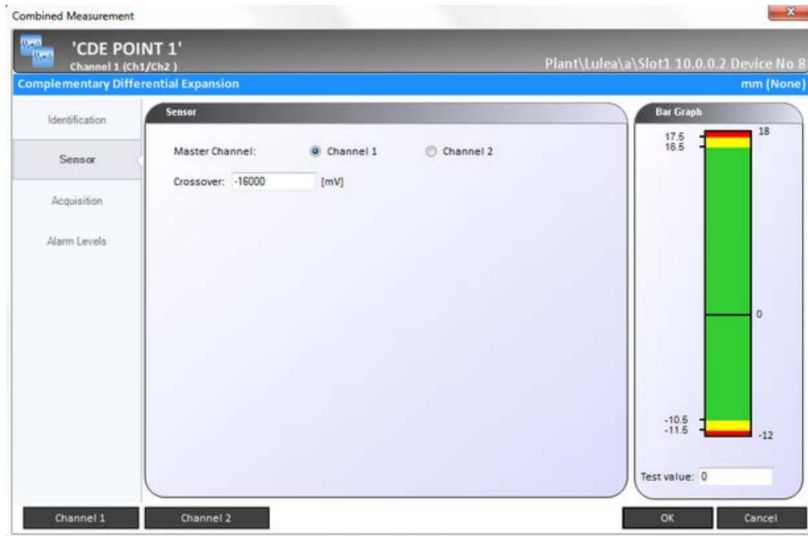
Figure 2 - 90. Combined Measurement Acquisition Setting.
