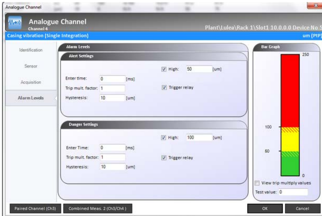
Figure 2 - 108. Setting the Alarm Levels.
