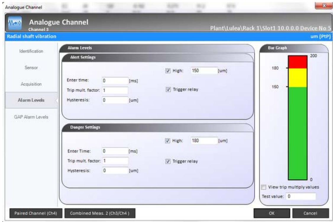
Figure 2 - 112. Setting the Alarm Levels.
