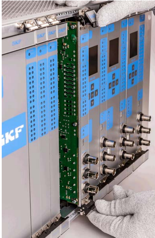
Figure 4 - 23. Demonstration of Ejecting a PRM.
