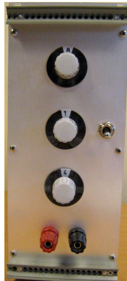
Figure 11-16: A SKF Cable Adapter for Cable Condition Test
