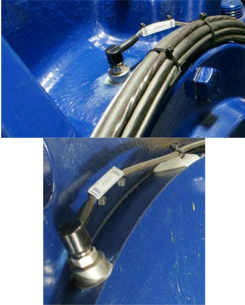
Figure 3 - 3. Examples of Attachment by Glue.
