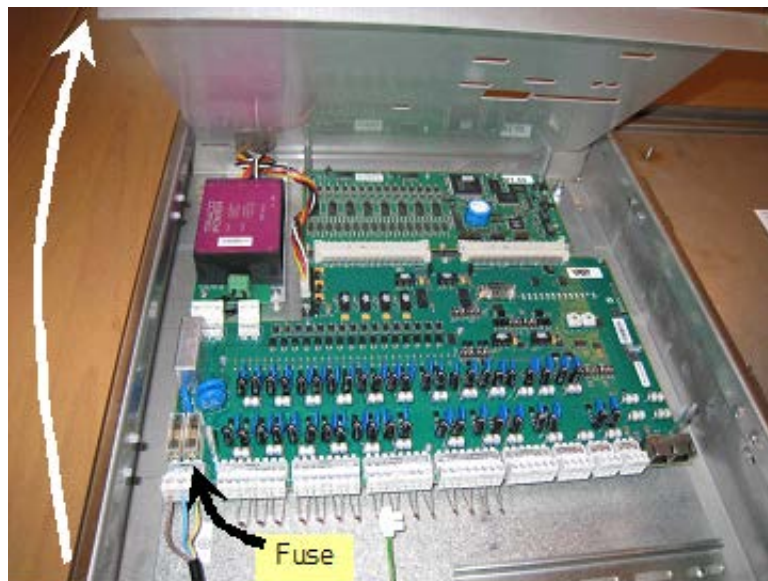
Figure 4 - 4. Lift the Front Panel and Remove.
