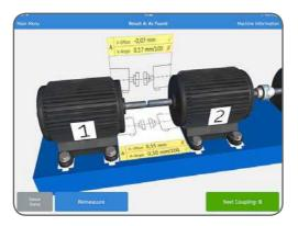
The values are compared with the selected tolerances and the symbols to the right, of the offset and angular misalignment values, indicate if the values are within tolerance.
