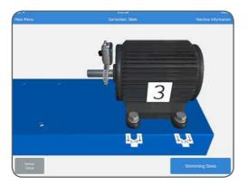
After the correction, or if no correction is needed, tap Shimming Done.
