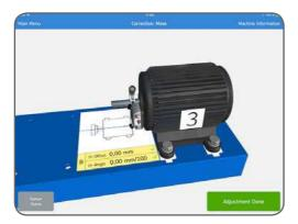
An animation shows the bolts being tightened down. Alignment is now complete and to confirm the result there is a need to re-do the measurement.
