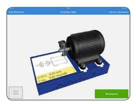
An animation shows the bolts being tightened down. Alignment is now complete and to confirm the result there is a need to re-do the measurement. Tap Remeasure.
