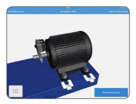
After the correction, or if no correction is needed, tap Shimming Done.
