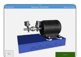
When the system senses that the shaft has again been rotated sufficiently, and has been left untouched for a short while, it will automatically record the  $3^{rd}$  measurement position.
