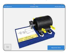
Move the machine according to the arrows and observe the offset and angular misalignment values that are updated continuously.
