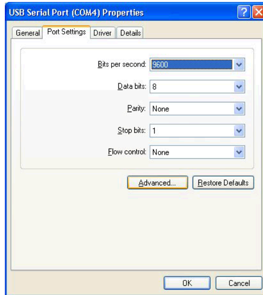
Figure 3 - 6. The USB Serial Port Properties Dialog's Port Settings Tab.
