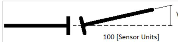
When /100 is selected the angular tolerance value entered ( $y$ ) must be in Sensor Units. In this example our Sensor Units are mm, so if we enter 0.08 (mm), this corresponds to an angular tolerance of 0.08mm / 100mm.
