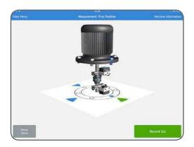
The display shows a simulation of the 90° rotation, of the Measurement units, to the second position. Now turn the units to this position.
