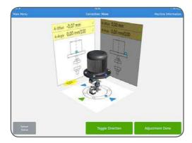
Alignment is now complete and to confirm the result there is a need to re-do the measurement. Tap Remeasure.
