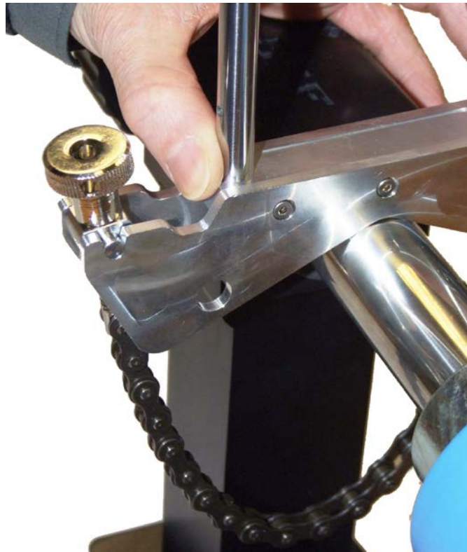
Figure 3 - 10. Attaching the Pivot to the V-Bracket.
