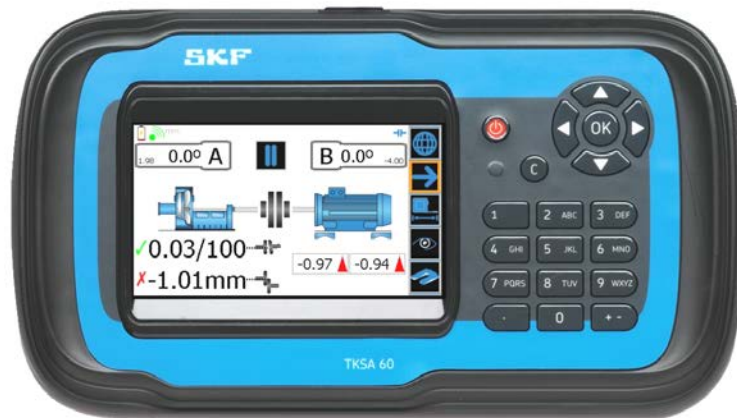
Figure 2 - 1. The TKSA 60 Display Unit.
