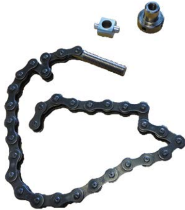
Figure 3 - 7. Chain, Pivot, and Knurled Knob.
