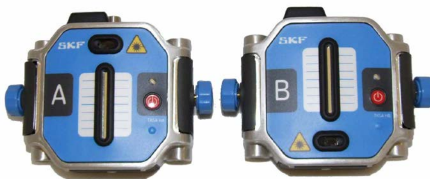
Figure 3 - 1. The TKSA HA and TKSA HB Measuring Units (Front).
