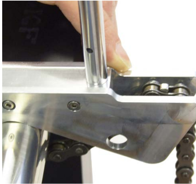
Figure 3 - 9. Attaching the Chain Assembly to the Anchor.
