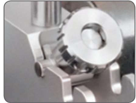
Make sure the rods are **firmly tightened** to the brackets before mounting the measuring units.
