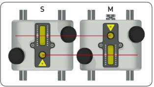
Adjust the laser lines to the center of the detectors. Start by vertically adjusting the Measuring Unit S on the rods. Use the laser adjustment knob on the Measuring Unit M. The sensor status of the App indicates the correct position.
