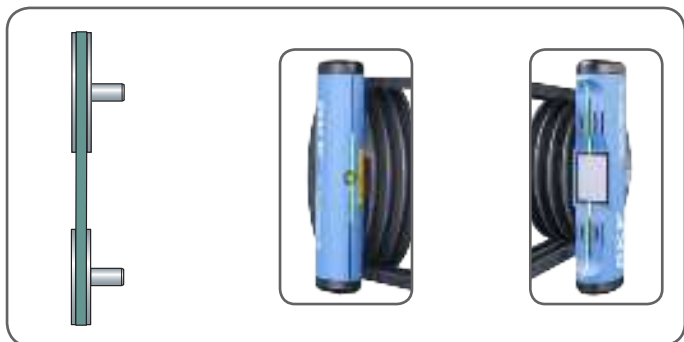
Figure 9 Pulleys perfectly aligned
