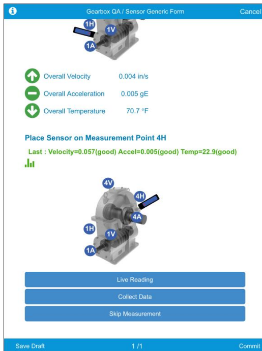
Figure 40 Vibration data: Continue taking readings
