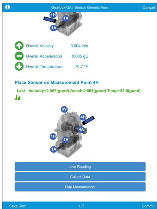
Figure 40 Vibration data: Continue taking readings
