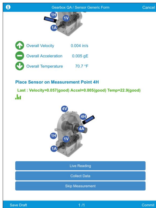
Figure 40 Vibration data: Continue taking readings
